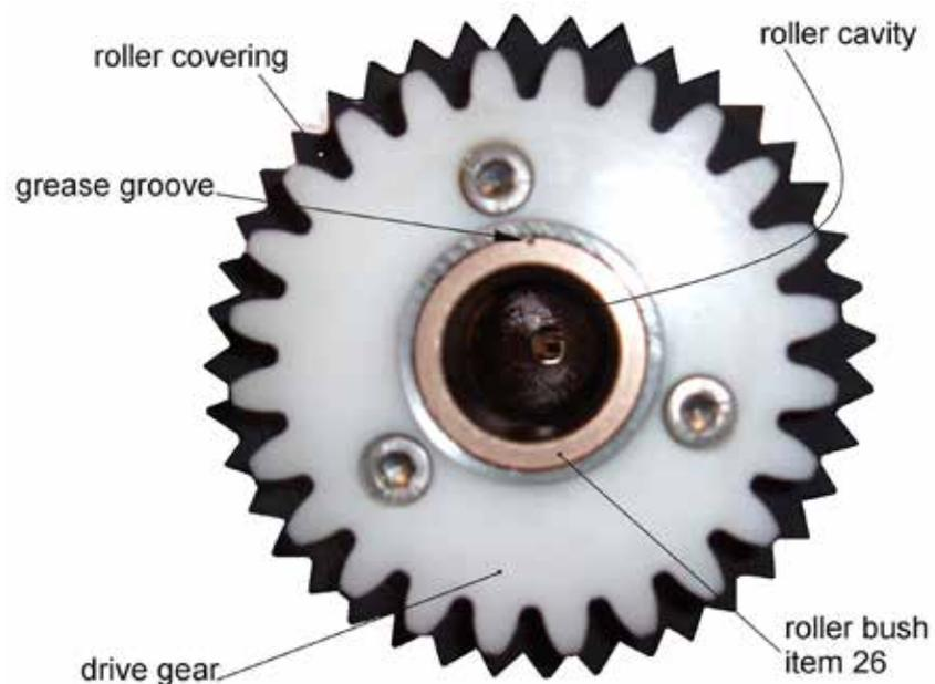
Roller shaft & support plates removed for clarity omitted for clarity.
